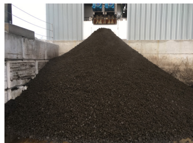
Daily volume of stackable solids produced by DVO Phosphorus Recovery System.
